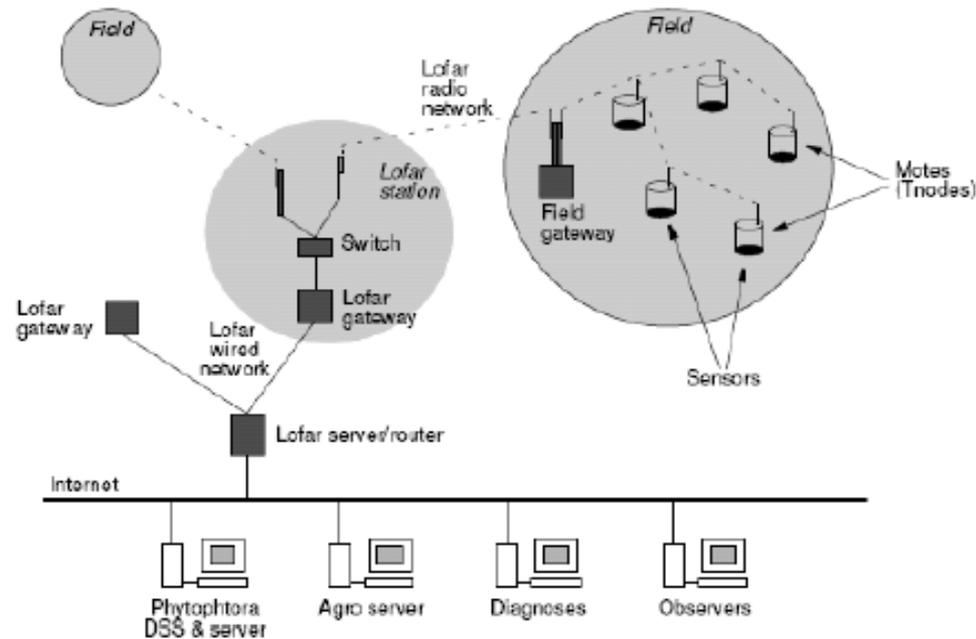
Sensor nodes send the gathered data via a wireless connection every 10 minutes to field gateways which send it to an ordinary PC for data logging (the Lofar gateway in the figure). The data is further transmitted to other servers for data analysis via a wired Internet connection. A decision support system maps the temperature distribution together with other information. Based on this information, farmers can take different actions and vary the amount of fertilizer and pesticide used.
